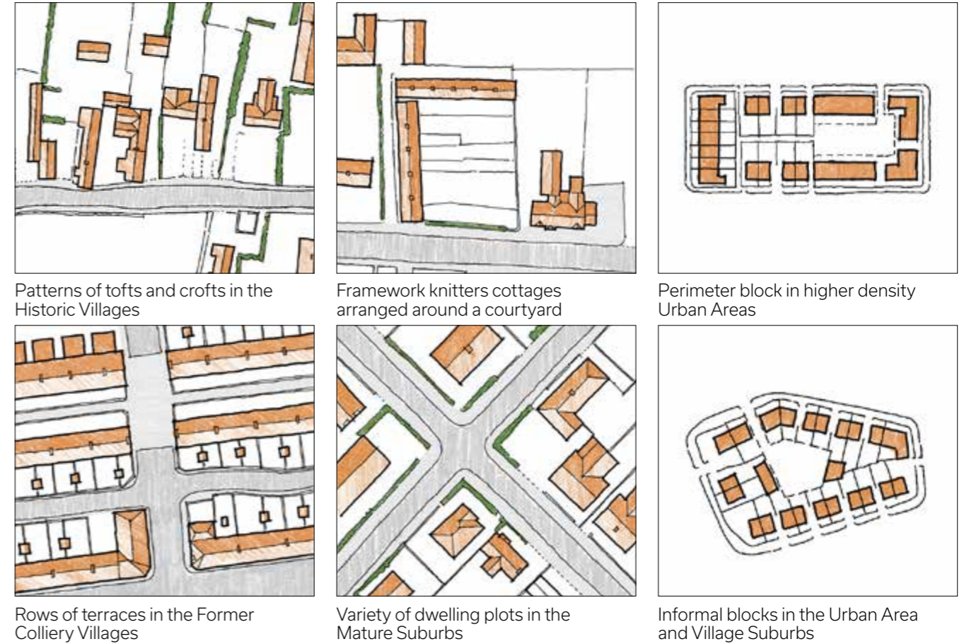
Figure 3: The patterns of built forms that can be found across settlements in the Gedling Borough that relate to the Historic Villages, Former Colliery Villages and Mature Suburbs in the Urban Area
