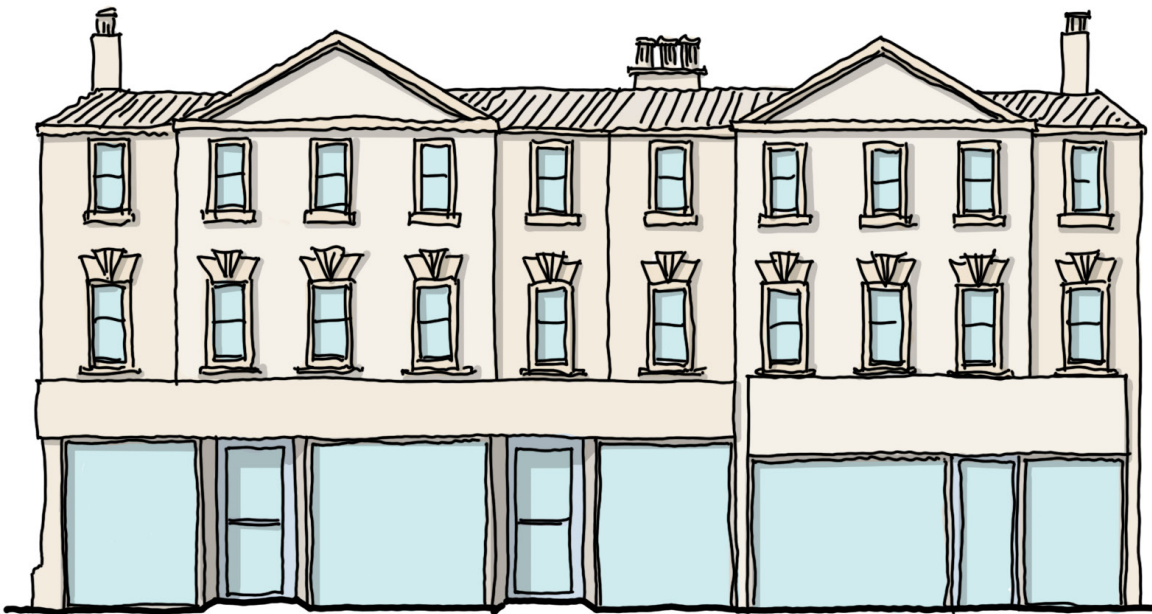
Poorly designed shopfronts do not respect the style, proportions and detailing of the rest of the building.
